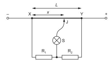
J is moved along XY to a point at which the lamp is off. This point is at a distance x from X.
